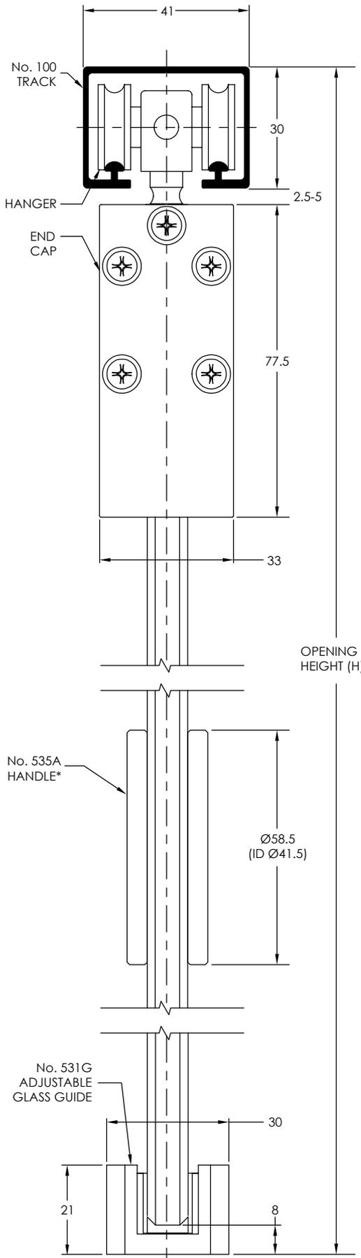
\* FOR No. 535G ROUND GLASS HANDLE, MACHINE A Ø50 HOLE TO FIT HANDLE
